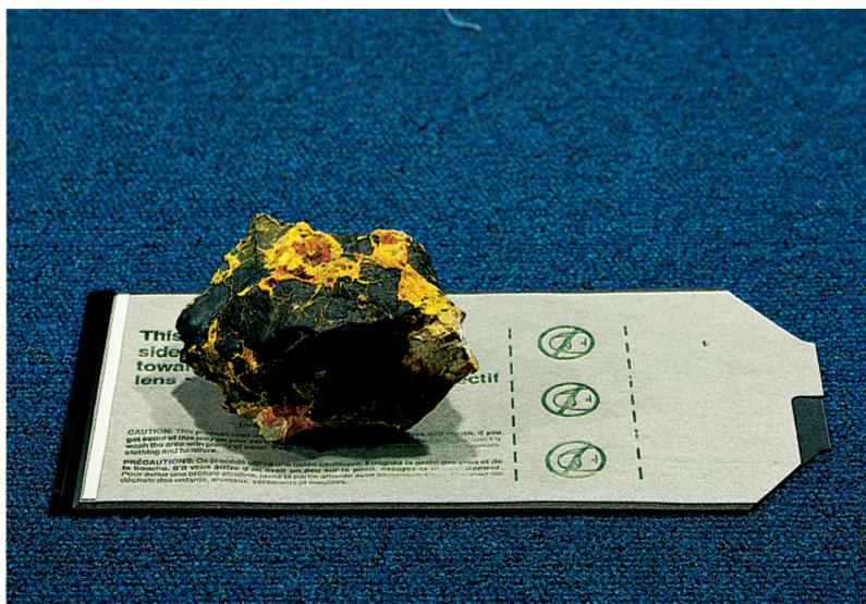
Figure O.1 (left) When a sample of \text{K}_2\text{UO}_2(\text{SO}_4)_2(s) is placed on photographic film, which is wrapped in opaque paper, the radioactive emissions pass through the protective paper and cause the film to appear as if it had been exposed to light. (right) A metal key that was placed below the sample blocked the emissions, so we see the outline of the key on the developed film.
