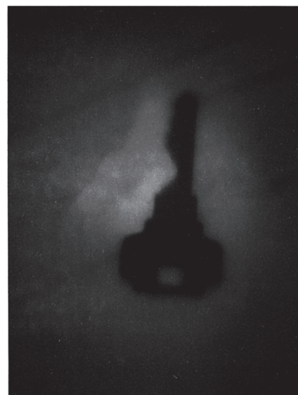
Figure O.1 (left) When a sample of \text{K}_2\text{UO}_2(\text{SO}_4)_2(s) is placed on photographic film, which is wrapped in opaque paper, the radioactive emissions pass through the protective paper and cause the film to appear as if it had been exposed to light. (right) A metal key that was placed below the sample blocked the emissions, so we see the outline of the key on the developed film.
