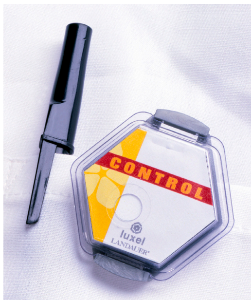
Figure O.5 Film badges, such as the one shown here, are worn by radiation workers and are routinely monitored to guard against accidental radiation exposure.
