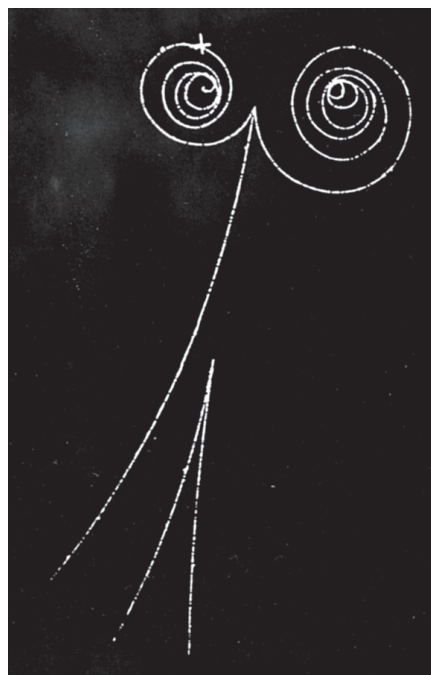
Figure O.3 An electron and a positron annihilate each other to produce two \gamma -ray photons. The reverse process also occurs; that is, a high-energy \gamma -ray photon can transform spontaneously into an electron and a positron, as seen in this photograph from a bubble chamber. Because it is uncharged, the photon leaves no track, but the electron and positron leave visible spiral tracks. An externally applied magnetic field causes the tracks to be spirals, and the opposite charges on the electron and positron cause them to spiral in opposite directions.
